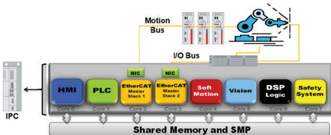
The ability to assign different functions to different cores that communicate via shared memory makes it easy to change out and control such things as different tools that are to be controlled by the vision system. The ability to assign different functions to different cores that communicate via shared memory makes it easy to change out and control such things as different tools that are to be controlled by the vision system.
