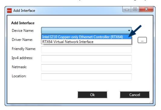
6. In the **IPv4 address** and **Netmask** box, enter the information to use with the selected NIC, and then click **OK**. For example, you can enter 192.168.1.6 for **IPv4 address** and 255.255.255.0 for **Netmask**. If you have more than two NICs installed on the same computer, make sure the IPv4 address of the selected NIC doesn't conflict with that of other NICs.
