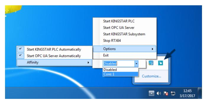
4. Click **Start KINGSTAR Subsystem**. After you assign the core, KINGSTAR Subsystem will run on that core every time you start the Subsystem.
