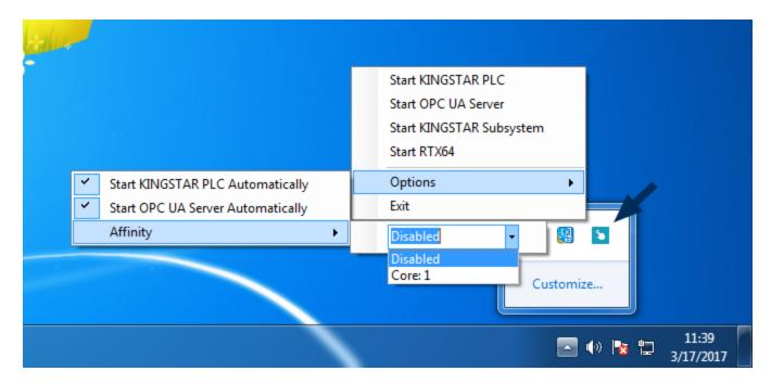
**Start KINGSTAR PLC**: Starts or stops KINGSTAR Soft PLC Runtime manually. It displays **Stop KINGSTAR PLC** after you start it. To run a PLC program, the KINGSTAR Soft PLC Runtime must be started. By default, it is started.
