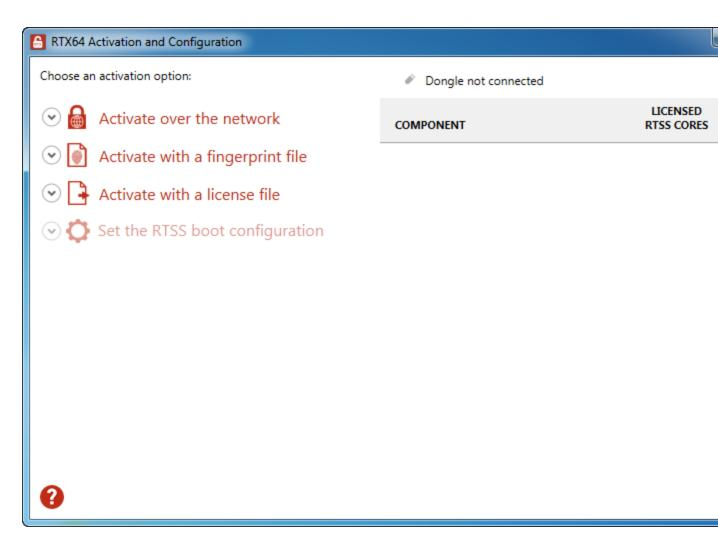
Click Activate over the network. Make sure your machine is connected to the internet with access to the IntervalZero license server. If a connection is available, you will see Connection established. If the connection is not available, make sure all network
