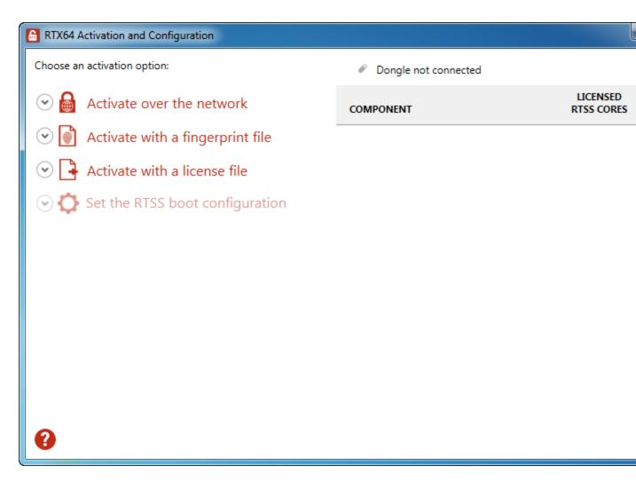
2. Click **Activate over the network**. If it doesn't connect to the IntervalZero license server, you'll see **Unable to establish a connection**. If the connection is available, you will see **Connection established**. For further details, see the section Activate over the internet.
