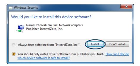
9. The RTX64 driver installs for the network adapter. Click **Close** after the installation is completed. The network adapter is now available for use with KINGSTAR.
