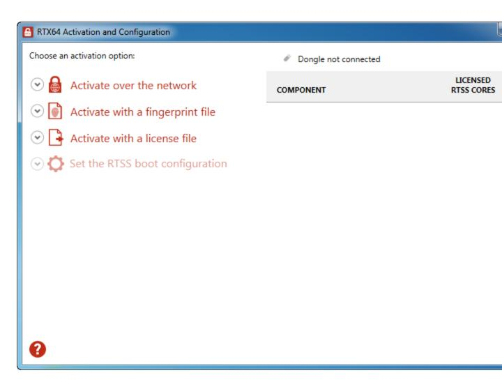
2. Click **Activate over the network**. Make sure your machine is connected to the internet with access to the IntervalZero license server. If a connection is available, you will see **Connection established**. If the connection is not available, make sure all network
