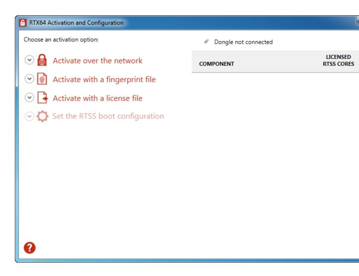
Click Activate over the network. If it doesn't connect to the IntervalZero license server, you'll see Unable to establish a connection. If the connection is available, you will see Connection established. For further details, see the section Activate over the internet.
