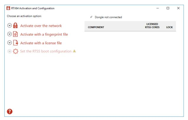
Click **Activate over the network**. Make sure your machine is connected to the internet with access to the IntervalZero license server. If a connection is available, you will see **Connection established**. If the connection is not available, make sure all network
