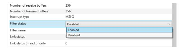
9. In the **Filter name** box, browse to the file ksio64filter.rtdll, which is in the <ksmDir>\bin (<ksmDir> is the location where KINGSTAR was installed). This will associate the KINGSTAR filter with the interface.
