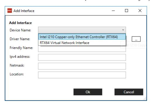
6. In the **IPv4 address** and **Netmask** box, enter the information to use with the selected NIC, and then click **Ok**. For example, you can enter 192.168.1.6 for **IPv4 address** and 255.255.255.0 for **Netmask**. If you have more than two NICs installed on the same
