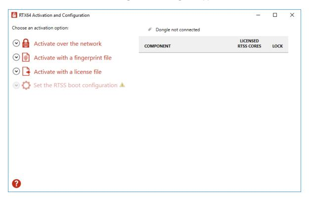
Click Activate over the network. If it doesn't connect to the IntervalZero license server, you'll see Unable to establish a connection. If the connection is available, you will see Connection established. For further details, see the section Activate over the internet.
