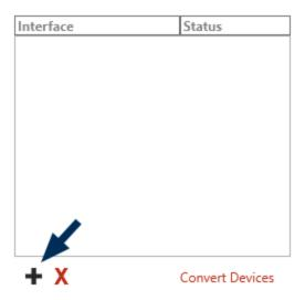
5. In the **Add Interface** dialog box, in the **Device Name** list, select a NIC that has RTX64 in its name. If the name of the NIC doesn't have RTX64, it means your NIC is not associated with KINGSTAR. See **Manually associate** a **NIC** to configure your NIC.
