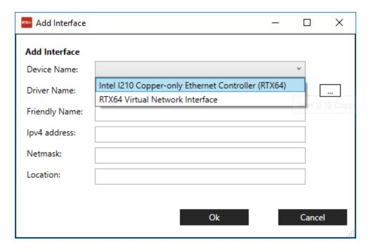
6. In the **IPv4 address** and **Netmask** box, enter the information to use with the selected NIC, and then click **Ok**. For example, you can enter 192.168.1.6 for **IPv4 address** and 255.255.255.0 for **Netmask**. If you have more than two NICs installed on the same
