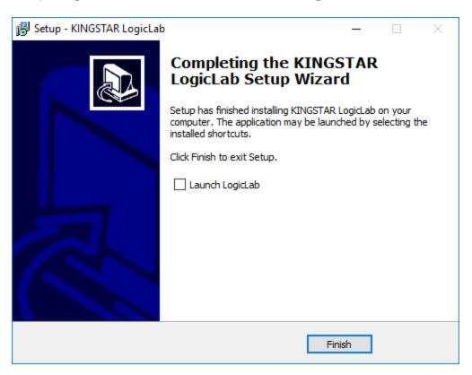
**NOTE:** KINGSTAR LogicLab can be installed on a local computer or remote computer. If you install KINGSTAR LogicLab and KINGSTAR PLC Runtime on the same computer, you can use **Scanbus** to add hardware to your PLC project automatically. If you install LogicLab individually on a computer, you can't use **Scanbus**, but you can download your PLC program to the computer that has KINGSTAR PLC Runtime installed and run it remotely. KINGSTAR PLC Runtime is incorporated in KINGSTAR Motion Runtime.
